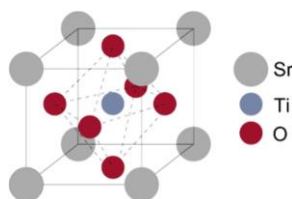
Fig. 1. Structure of the lattice of SrTiO_3 [20].
