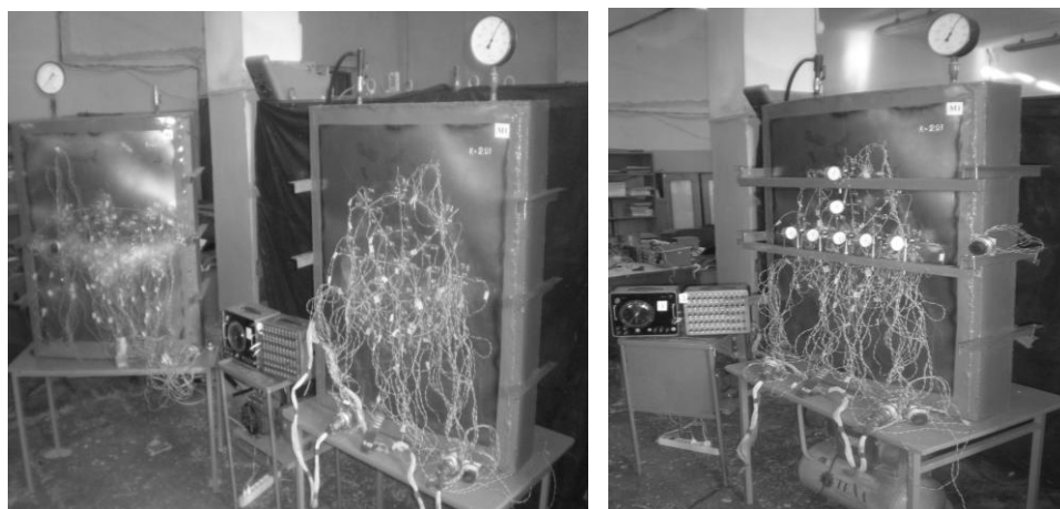
Figure 1 - General view of fragment model of the tank wall with dents
